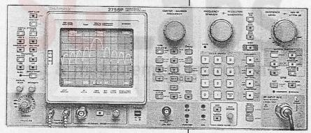
as Tek's WM490 Series, or the new WM780 Series (each WM780 Series mixer is individually calibrated). Signal sensitivity is an impressive -134 dBm. The 2756P is optimized for use in baseband through millimeter-wave measurements, where the ability to identify and process signal frequencies and amplitudes over wide dynamic ranges with high accuracy is critical.
